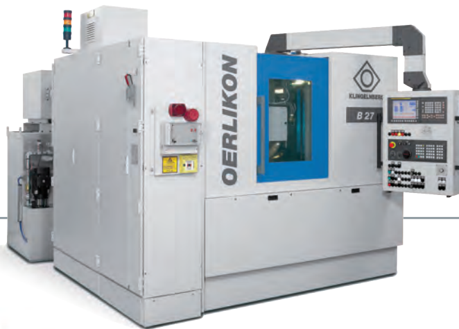
Oerlikon stick blade grinding machine B 27 for grinding stick blades for all bevel gearing types
