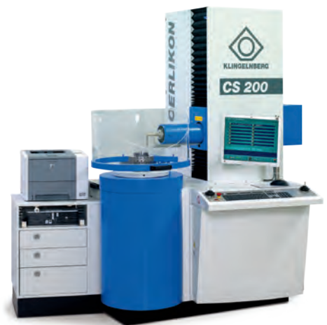
Oerlikon cutter head setting and checking device CS 200 for quick and easy setting of the cutter heads as well as for checking and documenting the cutter heads
