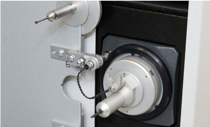
Fig. 1: Roughness probe and plug connector: In addition to the sensor technology, a precision swivel device is also integrated into Klingelnberg's extremely compact roughness probes. The roughness probes can therefore be operated on the adapter plate like the tactile styluses, and can be changed automatically. An especially convenient feature is the automatic plug-in.
