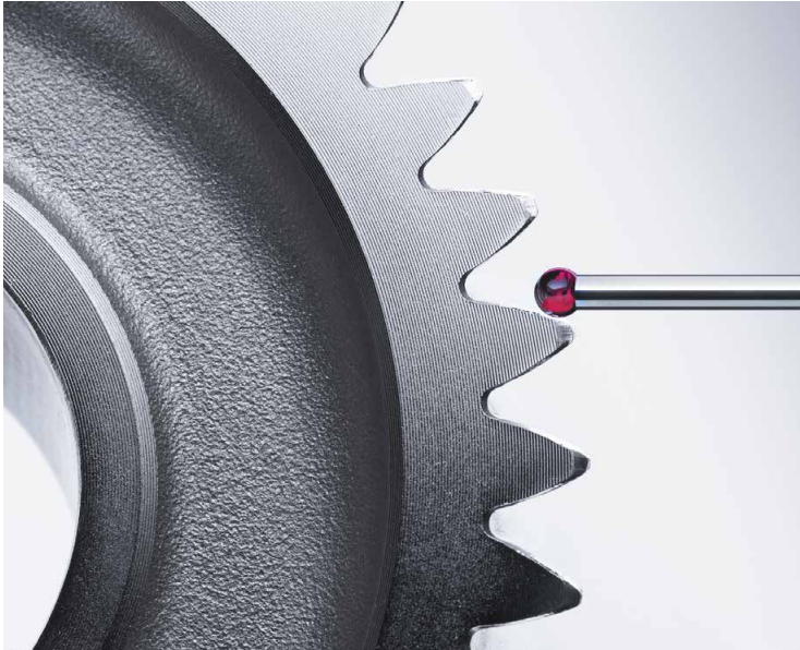
Analysis of the spectrum of waviness using the all-tooth measurement
