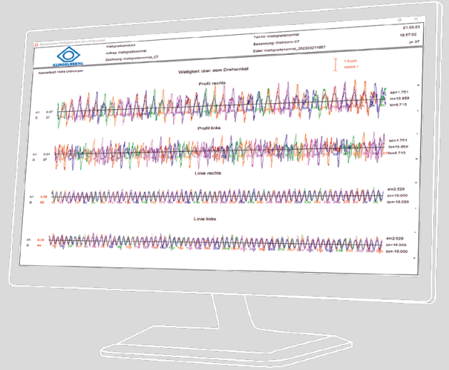
Evaluation of profile, flank and pitch using all-tooth measurement
